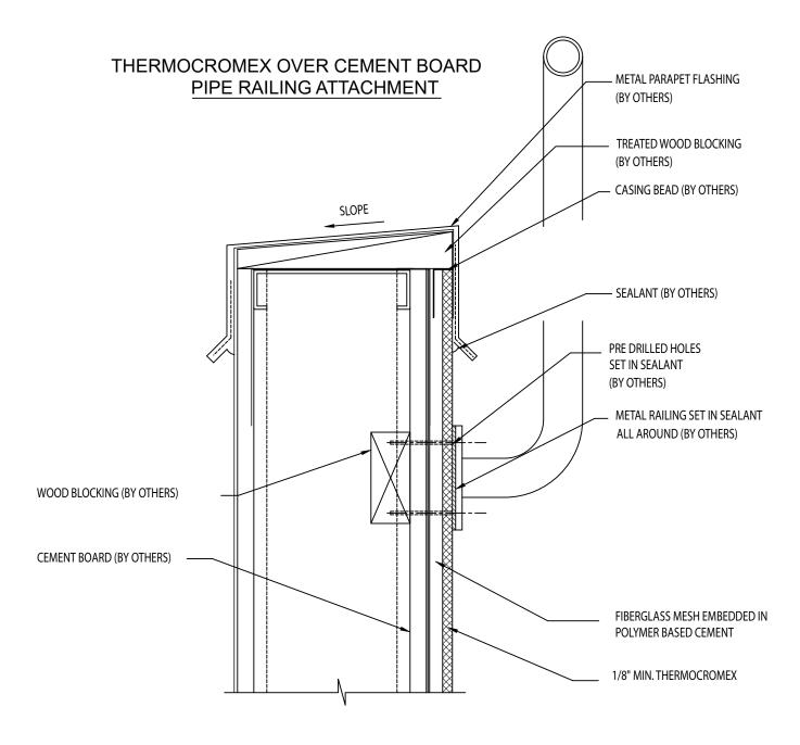
NOTE: All joints of cement board must be treated with 4" fiberglass mesh embedded in polymer based cement.
